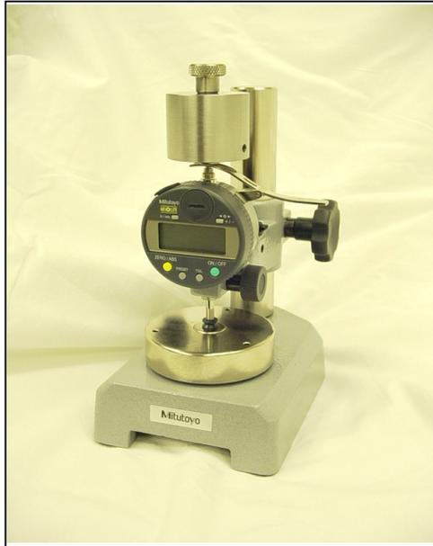
*Model 543 Dead-Weight Digital Indicator & Stand. Shown with Add-Weight, Lift Lever and Parallelism-Adjustable Anvil Option*
